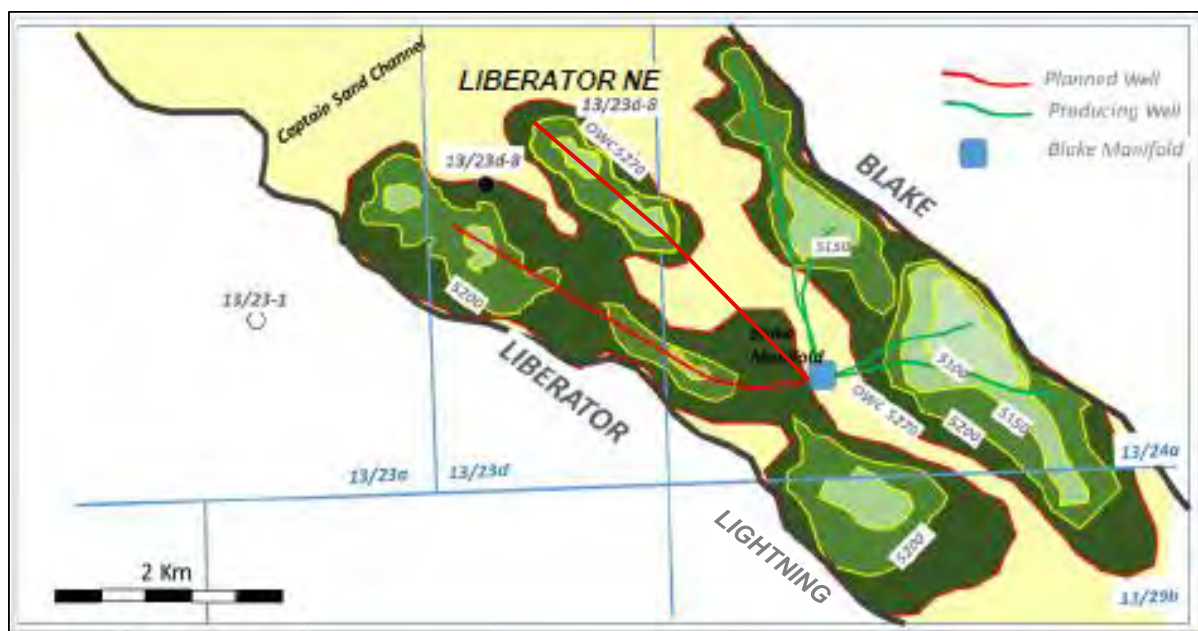
Figure 7: Schematic Illustration of Proposed Two-Well Development
